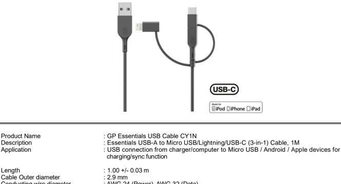
: AWG 24 (Power), AWG 32 (Data) Conducting wire diameter **Data Sync Function** : Yes Charging Function : Yes Rated Current : 5V/2.4 A, 9V/2A, 15V/1.5A (18W max.) Supported protocols : QC : 15 (W) x 7 (H) x 1000 (L) mm Product dimension Weight : 21g (approx.) Cable Sheath Material : TPĔ : CE Approval Compliance : RoHS Warranty Period : 12 months from ex-factory date
